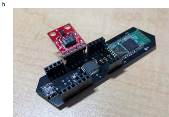
Fig. 3a. Layout for Clamshell V1. Fig. 3b. Test build for Clamshell V1.
